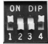
DIP SWITCHES SET TO '1001'
